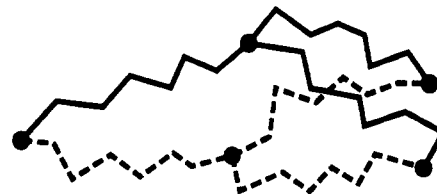
Figure 2. An internal wiggle, one of two fundamental Monte Carlo moves, consists of moving one spacer and its two daughters (initial and final configurations represented by solid and dashed lines, respectively) while holding the rest of the molecule in place.
